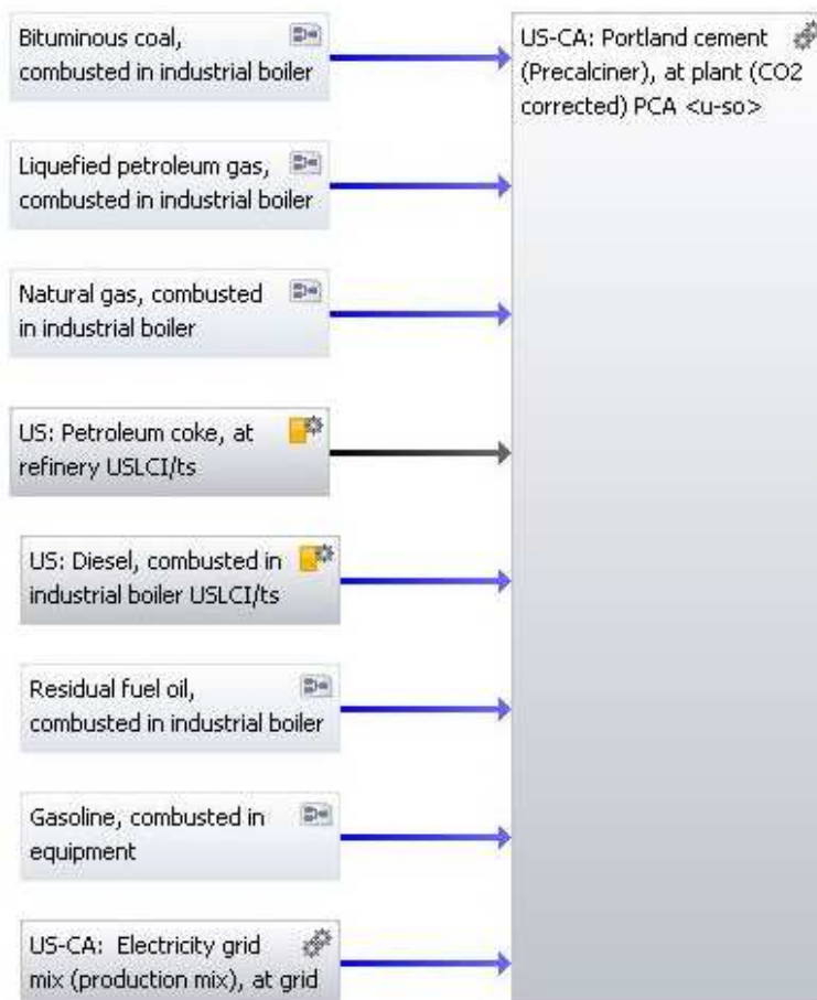
Figure 3.18: The model developed for cement production (precalciner method + CA electricity mix.)
