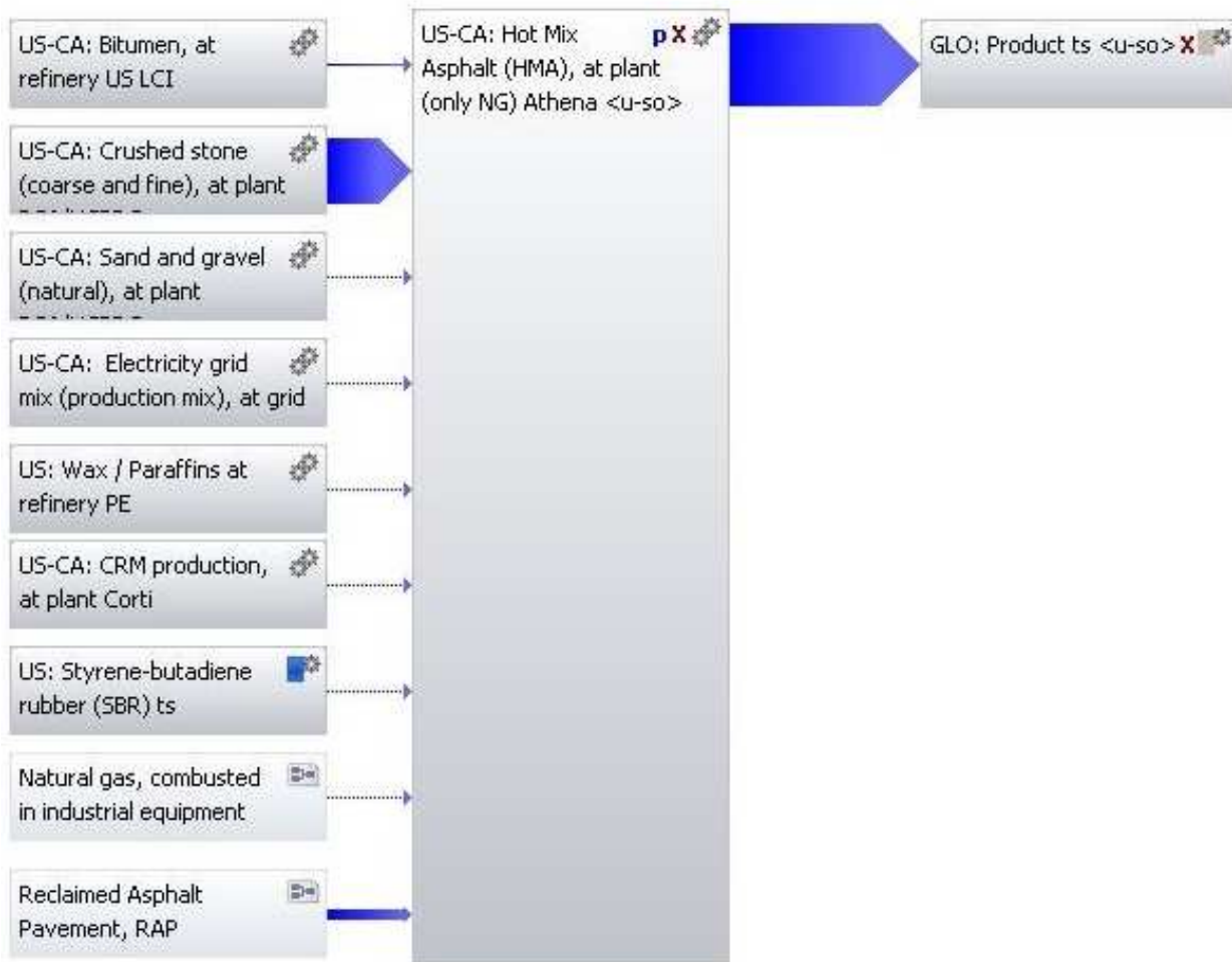
Figure 3.35: The model developed for HMA (the mix design can be modified)
