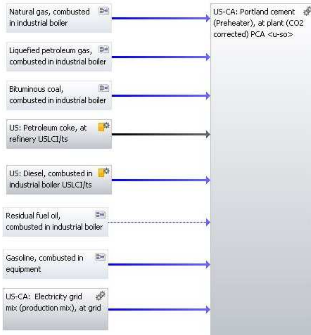
Figure 3.20: The model for cement production (preheater method + CA electricity mix.)
