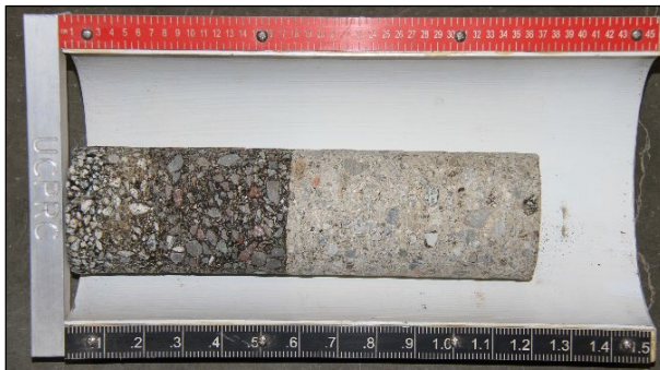
Figure 2.43: Concrete beneath asphalt layers (composite pavement).
