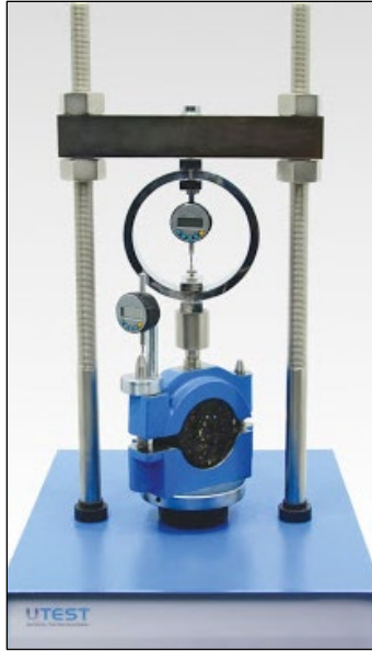
Figure 5.2: Marshall Stability Test.
