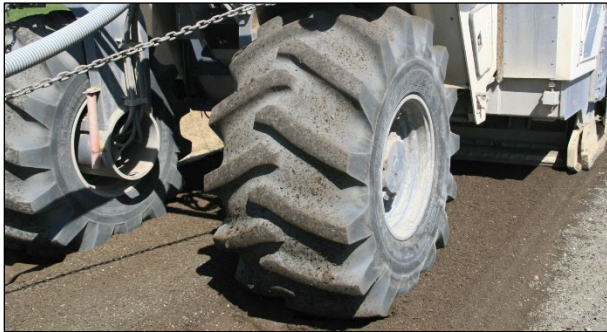
Figure 6.39: Normal tire condition when nozzles are functioning correctly (FDR).
