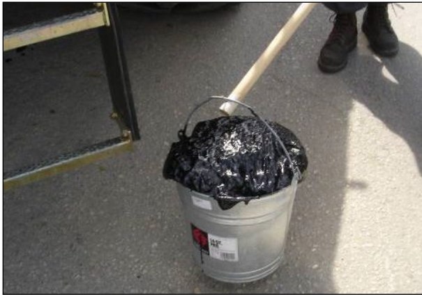
Figure 6.25: Checking binder foaming characteristics after tanker change.
