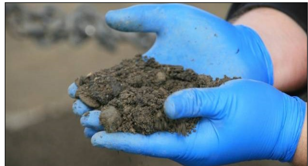
Figure 6.35: Checking material consistency and gradation (FDR).
