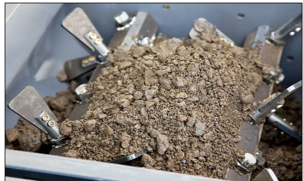
Figure 5.7: Pugmill mixer used for all mix designs to replicate recycler mixing.
