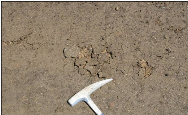
Figure 6.102: Delamination after blading thin lifts of material during grading (FDR).
