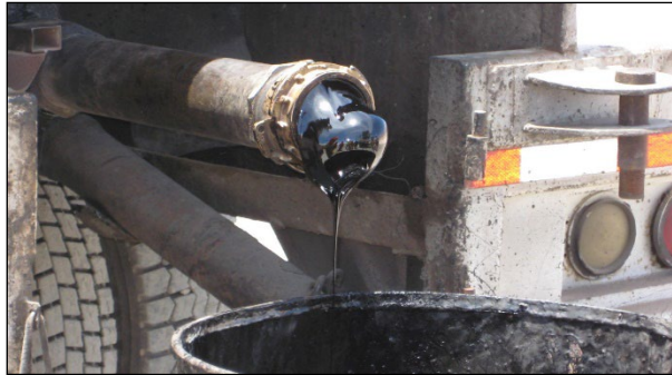
Figure 6.48: Cold plug in the asphalt feed connection of a binder tanker.
