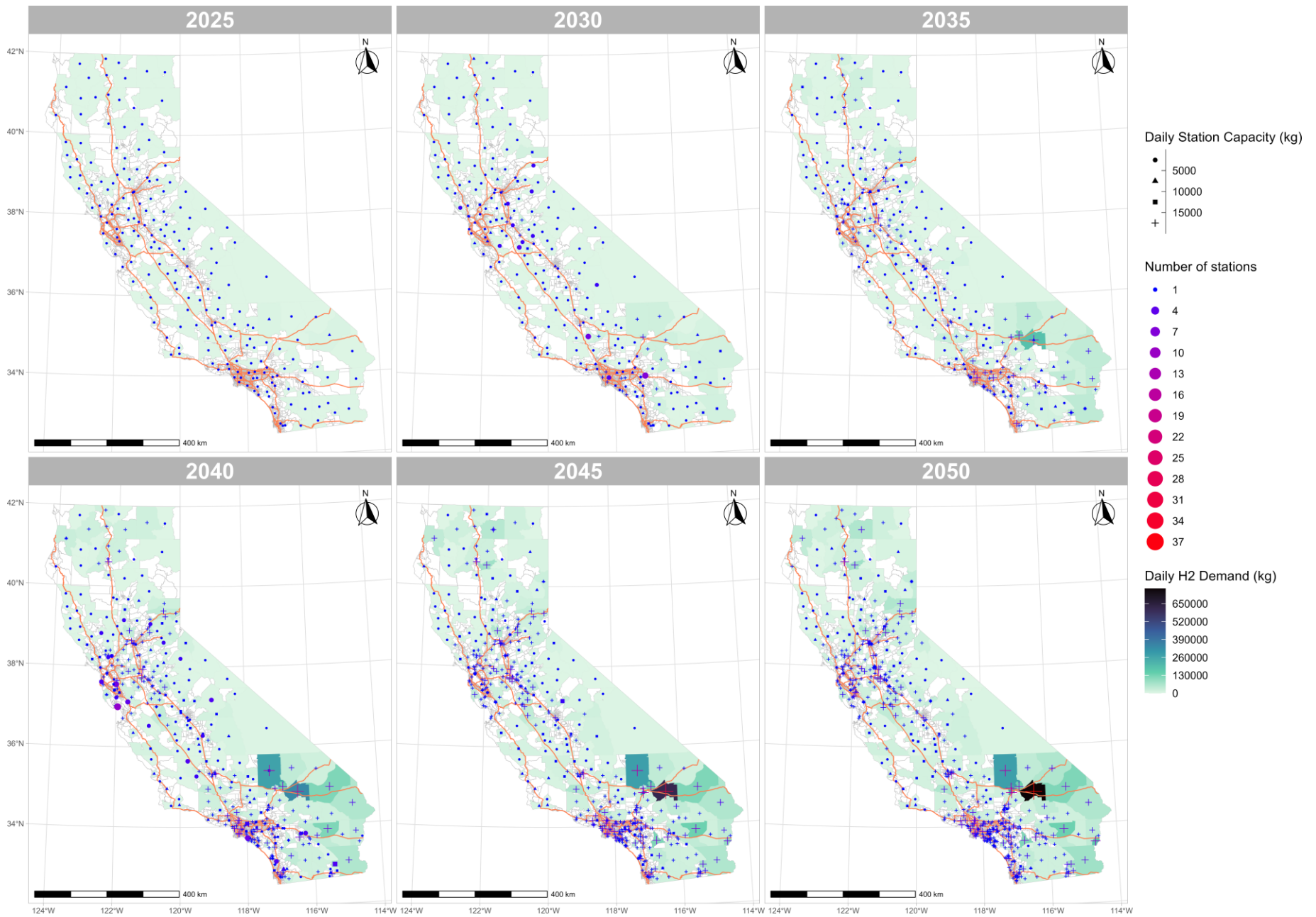
Figure 25. Number and daily capacity of stations, and refueling demand, by TAZ in High case
